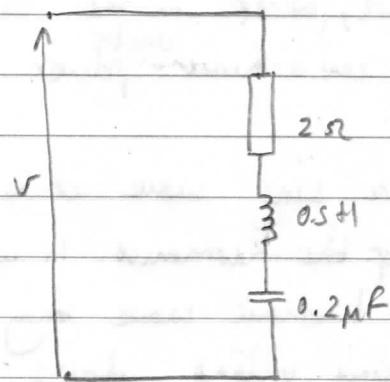
fundamental has a maximum value of 400V. The 3rd harmonic has a maximum value of 10V. Determine (a) The fundamental frequency of the 3rd harmonic (b) The maximum value of the fundamental and third harmonic components of current.
